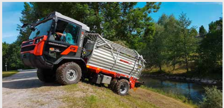
The Muli T10 X is gentle on the ground with a high ground clearance of 400 mm.
